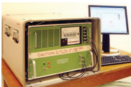
FIGURE 1: A modern portable Digisonde, with screen showing an ionogram.
